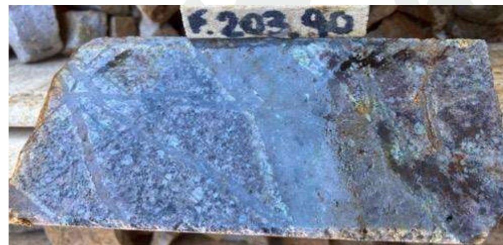
Hole PIU03: Multi-phase quartz veins stockworks and Cu oxides in potassic altered inter-mineral diorite porphyry (203.90m)
