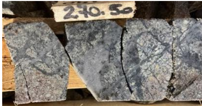
DDH PIU01: Multi-phase quartz veinlets in potassic altered inter-mineral diorite porphyry (270.5m)
