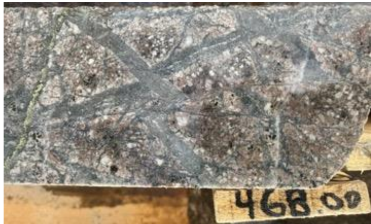
DDH PIU02: Multi-phase quartz vein stockworks in mineralized primary porphyry (468m)
