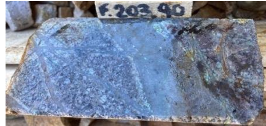
DDH PIU03: Multi-phase quartz veins stockworks and Cu oxides in potassic altered inter-mineral diorite porphyry (203.90m)
