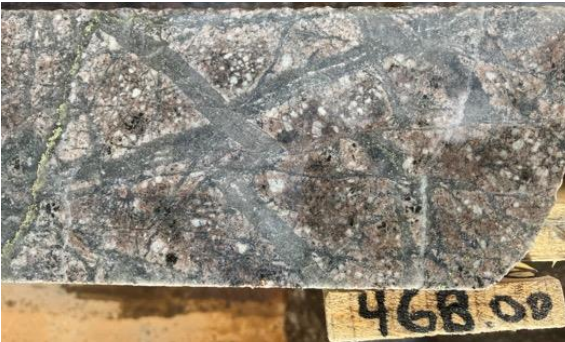
Hole PIU02: Multi-phase quartz vein stockworks in mineralized primary porphyry (468 m)
